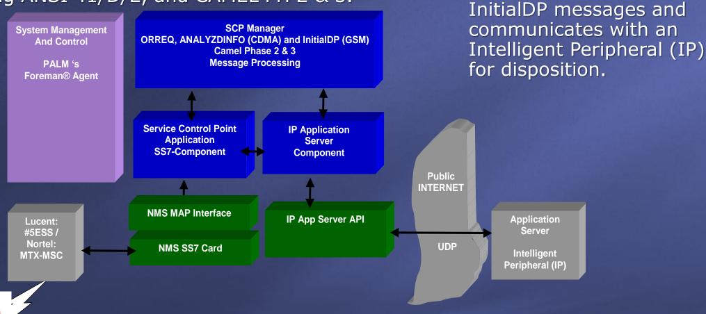
The system is implemented on Linux ES (Enterprise Server) using NMS (Natural Microsystems) SS7 boards and has been successfully integrated with a Lucent #5ESS switch, as well as Nortel CDMA and GSM switches. Cantata MSP 1010 version integration with Alcatel underway.
